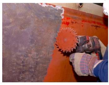
This movement ensures that the tips clean the surface perfectly, removing all contaminants and other old coatings. The hammer effect creates no heat, so tough materials such as tar, adhesives and sealants will be easily removed, and the Tercoo doesn't clog up.
